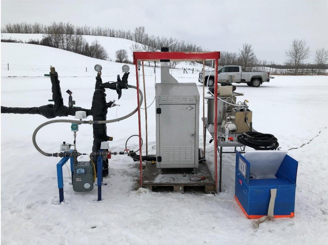
Figure 3: Metan CMAS-1S Catalytic Combustor at the Field Test Site
